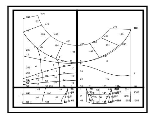
The model will be divided into four quarters. The surfaces in each of the quarters will be used to construct a single, composite surface for that quarter of the model. The four newly created composite surfaces will then be meshed and equivalenced, creating a single, fluid, consistent mesh which can be used for purposes of analysis.
