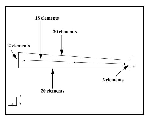
Curve List: select associated curve **Apply** Number of Elements: 2 shift click to select Curve List: left and right edge Apply 20 Number of Elements: Curve List: shift click to select top and bottom edge **Apply** Action: Create Object: Mesh
