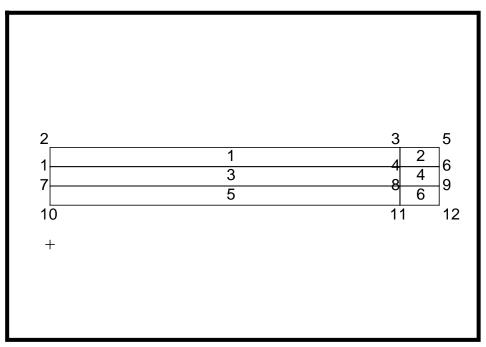
The flow of fuel within the nozzle will be modelled with advection bars. Create the two curves where the bars will be placed. Change the *Action*, *Object*, and *Method* to **Create/Curve/XYZ**. For the first curve set the *Vector* and *Origin Coordinates List* to, <**4.5 0 0**> and **[0 0 0]** respectively.
