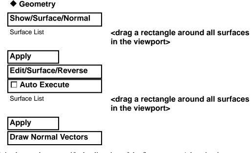
It is also prudent to verify the direction of the flow stream. Advection in an element flows in the local node 1 to node 2 direction. Unless reversed, the element local node 1/node 2 direction will follow the parent curve C1, or parametric, direction. Hence, it is sufficient to verify the C1 directions of Curve 1 and Curve 2. There is a toggle for displaying geometric parametric directions in **Display/Geometry**. Curves have only one parametric direction
