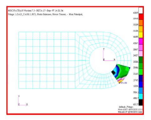
6. Convert the stress tensor results to the scalar  $\sigma_{xx}$ , and create a fringe plot of the scalar with respect to the cylindrical coordinate system you created when building the clevis model. Plot the results on all elements.
