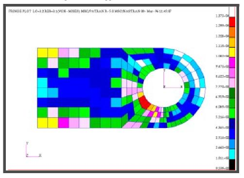
Filter Display 5. Create a fringe plot of the maximum principle stress for elements 1 through 20 only.
