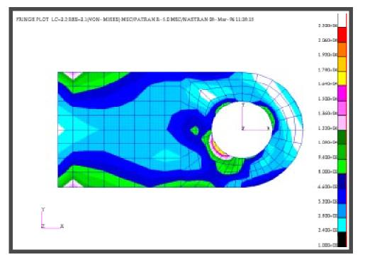
4. Render an element fill plot of the Von-Mises stresses.
