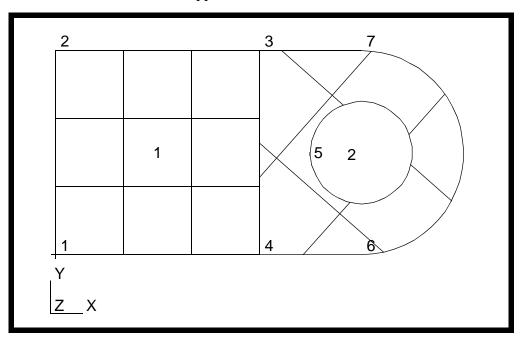
5. Mesh the simple surface (green) using the isomesher, and the trimmed surface (magenta) using the paver. Then extrude the mesh through the thickness as is appropriate.
