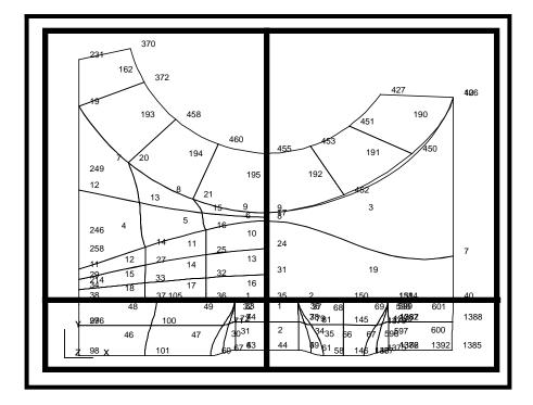
The model will be divided into four quarters. The surfaces in each of the quarters will be used to construct a single, composite surface for that quarter of the model. The four newly created composite surfaces will then be meshed and equivalenced, creating a single, fluid, consistent mesh which can be used for purposes of analysis.
