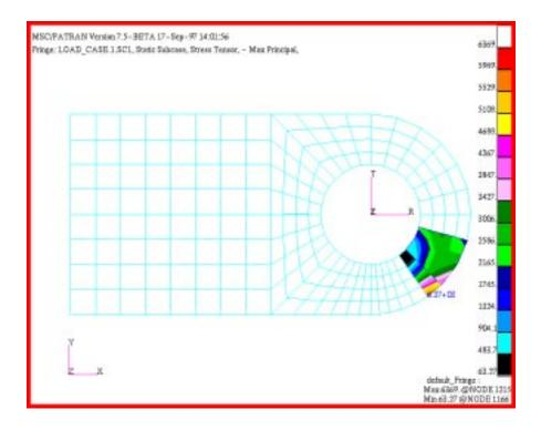
7. Convert the stress tensor results to the scalar  $\sigma_{xx}$ , and create a fringe plot of the scalar with respect to the cylindrical coordinate system you created when building the clevis model. Plot the results on all elements.
