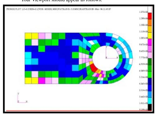
6. Create a fringe plot of the maximum principle stress for elements 1 through 20 only.
