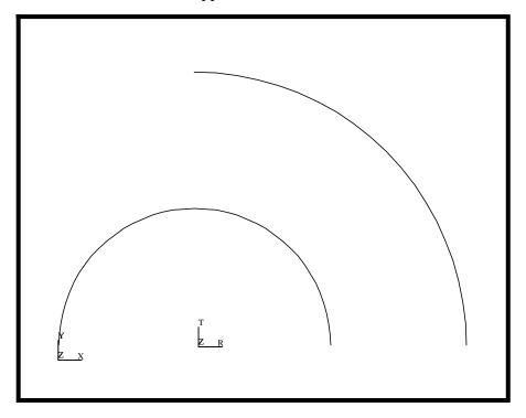
5.You have now created all the curves that you will need to complete your clevis model. Next, you will create the necessary surfaces for the model. You will start by creating a 4x2 Surface that defines part of the upper half of the clevis body.
