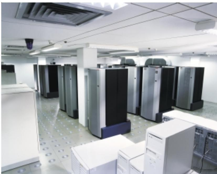
Parallelrechner IBM RS/6000 SP-SMP
