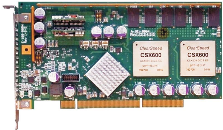
Abb. 1: Das ClearSpeed Advance Accelerator Board.
